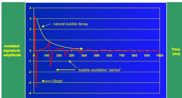
This signature shows the first, or primary, positive pressure pulse due to the initial expansion of the bubble. The following negative pulse, referred to as the “ghost”, is due to the reflection of the initial pulse at
